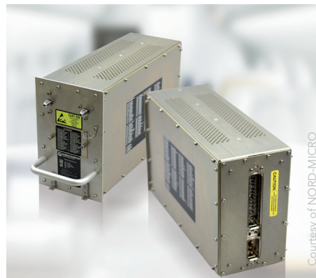
Avionic Bay/Data Acquisition
