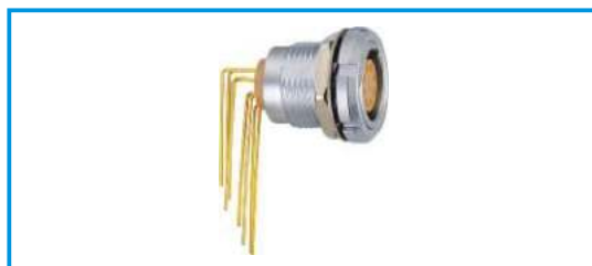
ZCG Fixed socket with two nuts, key (G) or keys (A... F) with elbow (90°) contact for printed circuit (back panel mounting)
